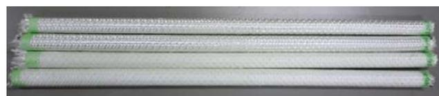
Fig.1 Resin impregnated glass fiber pipe 2200TEX
