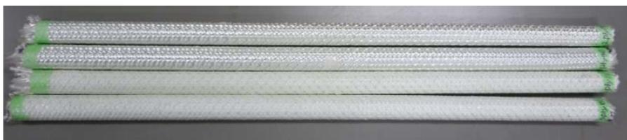
Fig.1 Resin impregnated **glass fiber(GF)** pipe 2200TEX Top 2: 2PLY, Bottom 2: 3PLY
